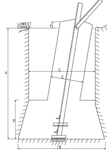
MAX. UPLIFT/ LEG = 54121kgs =530.93kN MAX. COMP/ LEG = 60076kgs =589.35kN MAX. TRANV. SHEAR/ LEG = 4,642kgs =45.54kN MAX. LONG SHEAR/ LEG = 4,126kgs =40.48kN VOLUME OF CONCRETE/ LEG = 8.8m<sup>3</sup>
